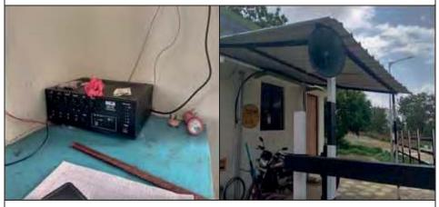
*Figure 2.22: SWR: Honey Bee Sound Device installed (without Honey Bee Sound) at L.C. Gate location Km.529/4 in Hubballi-Londa Section*
